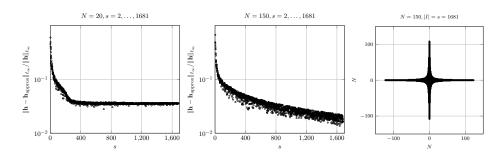
FIG. 6.4. Relative approximation errors  $\|\mathbf{h} - \mathbf{h}_{approx}\|_{\ell_{\infty}}/\|\mathbf{h}\|_{\ell_{\infty}}$  calculated by the spare FFT algorithm for the error function transformation with  $\boldsymbol{\eta} = \mathbf{1}, s = 2, \dots, 1681$  and the refinement N = 20 on the left and N = 150 in the center. The automatically constructed frequency set I for N = 150, s = 1681 is shown on the right.
